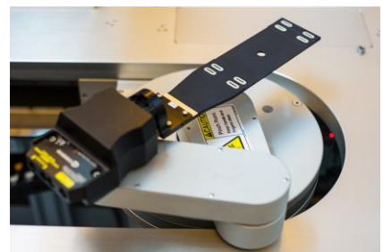
Pick and place robot for wafer handling with slot scanner
