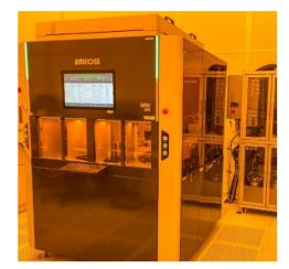
amcoss amc 2000 for fully-automatic, simultaneous coating and developing of wafers and substrates with varying diameters.
