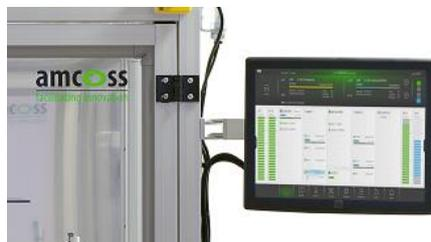
// Our intelligent **ams PILOT** software also controls processes in the **amv 200** and is being used to write recipes. As standard, a rotatable industrial PC with touchscreen and SECS/GEM interface is used to operate the machine.
