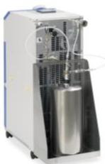
// An optional tray for the placing of the external DI cartridge, mounted on the backside of the chiller is available.
