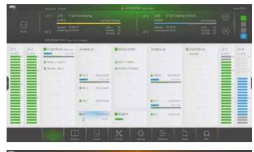
Log-function for informative reporting: The integrated log file consistently generates extensive machine reports for all production lots instead of just producing simple error logs.
