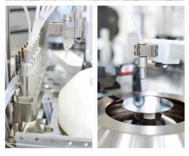
Solvent module for lift-off or resist-strip with innovative position-ing arm with single-nozzle grip. Only one nozzle at the time is being carried, which holds two major advantages: on the one hand there is no particle build-up caused by friction because only one tube at the time is being moved. On the other hand, all nozzles not required for the moment remain within the drip pan which prevents the tip of the nozzle from drying out and impedes delayed dripping onto the substrate.
