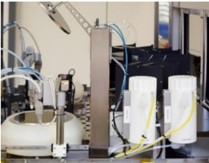
The system consists of a sensor-controlled reservoir and a suck-back dispense valve. The reservoir supplies the dispense valve which is mounted near the nozzle. The resist volume is set by pressure and trigger time.
