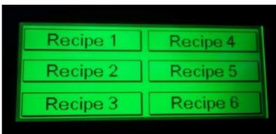
// 99 program recipes can be selected and adjusted (nominal temperature and processing time) directly on the integrated touch screen.
