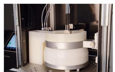
// Developer module with high splash ring for spray and puddle developing.
